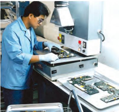
We're equipped with the latest BGA rework systems, and our staff of engineers and operators possess the knowledge and skills needed in the intricate world of BGA technology. A wide variety of services are offered, including:
